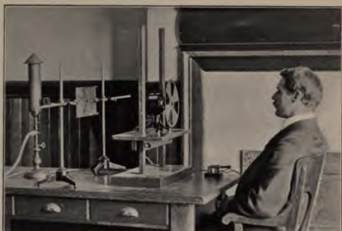
FIG. 1.—Apparatus for determining the most rapid succession of light sensations.
